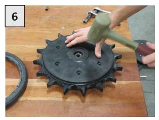
Align bolt holes and install the other hub half onto the bearing and tap back together with rubber mallet.
