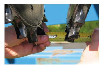
In high contour planting and turning on side hills, install the Furrow Cruisers in the front holes and widen them to approximately 1½ inches apart. This will help in keeping the spike out of the furrow and on the sidewall.
