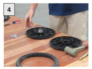
Remove the rubber wheel and lay the split hubs flat.
