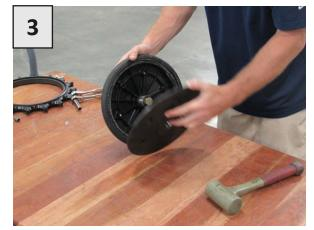
Continue to tap the bolt and pull apart. Do not attempt to pry the wheel apart with a screwdriver or you may damage the hubs.
