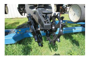
For optimal performance, Furrow Cruisers should be run in pairs.
