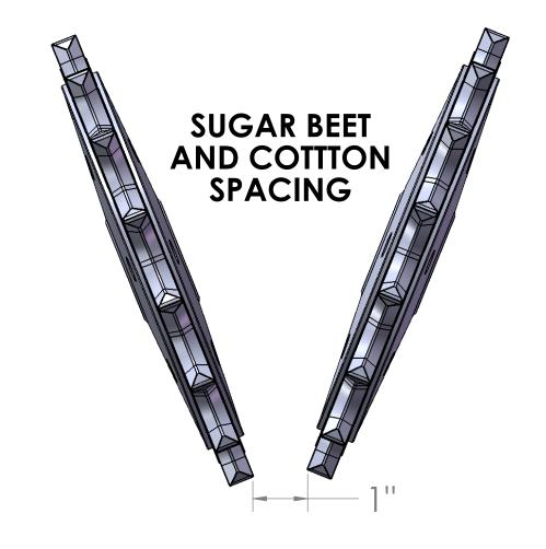
JOHN DEERE 7200 AND 7300 SERIES PLANTERS CAN ONLY FIT ONE SPACER WASHER IN BETWEEN THE WHEEL AND TAIL PIECE. THIS WILL ALLOW 7/8" TO 1 1/8" CLEARANCE BETWEEN THE WHEELS
